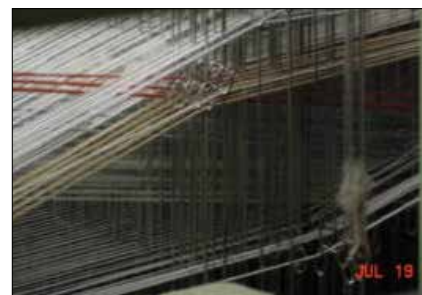
Detail of shed area of a mechanical loom.
