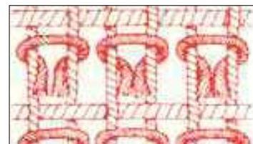
Symmetrical knots on a single wefted foundation.
