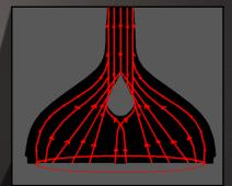
Sharp Shooter: Leading-Edge Design Allows for Uniform Laminar Airflow & Suction Throughout **Entire Length of Wand Head**
