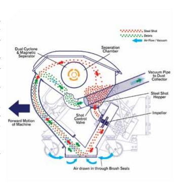
Accurate control of the shot blast pattern and the degree of removal or texture created is controlled using various machine settings and operational practices. These include:
