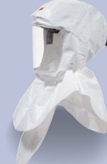
3M™ Hood Assembly S-657 Similar to S-655. The S-657 uses a double shroud design for its respiratory seal; wearers can select between seal designs based on their personal preference. The users wear the S-657 by tucking its inner shroud into a shirt or protective coverall, which allows excess air to be channeled over the body, providing additional comfort.
