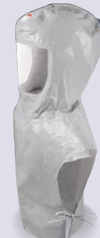
3M™ Hood Assembly S-857 Similar to the S-657 but made with Kappler™ Zytron™ 200 and sealed seams. Features a double shroud design for its respiratory seal. Both the S-855 and S-857 hood assemblies include ties to help keep the shroud in place.
