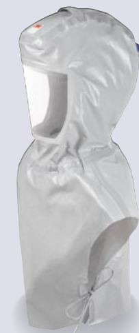
3M™ Hood Assembly S-855 Similar to the S-655 but made with Kappler™ Zytron™ 200, a polypropylene fabric with a multi-layer barrier film. The S-855 Hood Assembly also features sealed seams, making it suitable for environments where liquid splash hazards are present. Features a comfortable, knitted inner collar.
