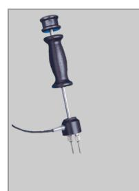
The industry standard for lumber and woodworking, this electrode allows you to determine moisture gradients. The contact pins that come with the 26-ES have insulated shanks so that only the tips are exposed. The pins make contact with the wood fiber only at their uncoated tips and provide much more accurate readings of moisture content at various levels of penetration. Knowing that the board is not uniform, you can use the pins to determine the drying pattern.
