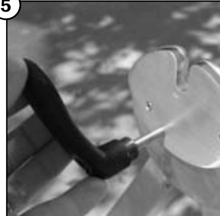
Locking levers can be stored on the fan stand by screwing them into the mounting holes in the spacer plate.
