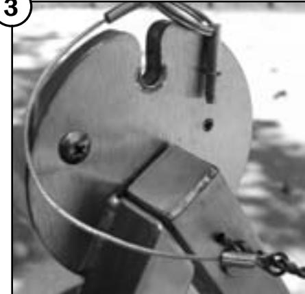
Drill out the rivets which secure the wire tethers to the fan stand. Discard wire tethers. These are not used with your Phoenix Axial Air Mover.
