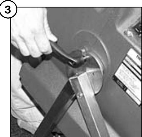
Aim the air mover for desired airflow direction and finger-tighten the locking levers.
