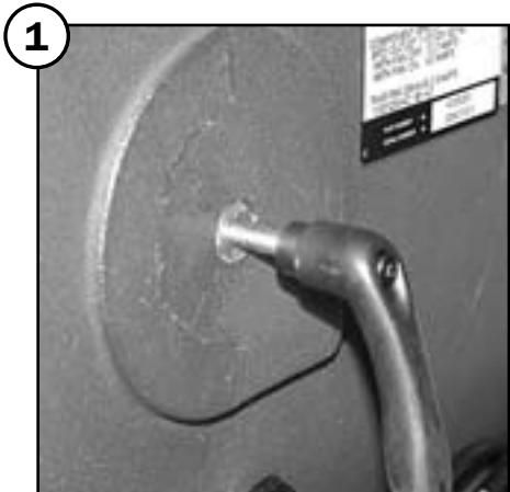
Screw both locking levers into the mounting lugs on either side of the air mover approximately 1/4".
