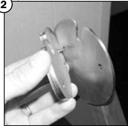
Attach one spacer plate to the inside surface of the mounting plate on both sides of the stand as shown.
