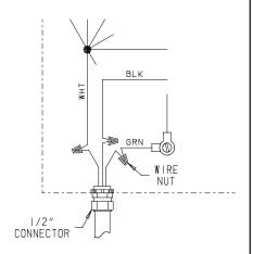
Figure 1: Hard Wiring the HI-E Dry 195
