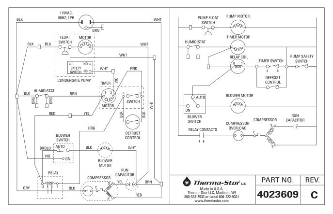
Figure 4: Electrical Schematic of HI-E Dry 195
