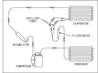
Figure 3: Refrigeration system of HI-E Dry 195
