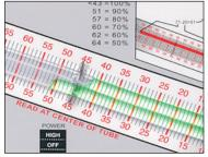
The built-in manometer provides precise measurement of air-flow through the HEPA filter and aids in determination of HEPA filter replacement intervals.
