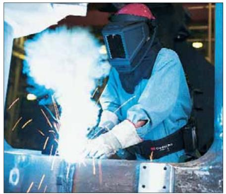
A PAPR is a powered air purifying respirator system that uses a fan to deliver filtered air into a hood, helmet or full facepiece. There are many different PAPR configurations available. Depending on the working environment, select the PAPR style that best meets your needs.
