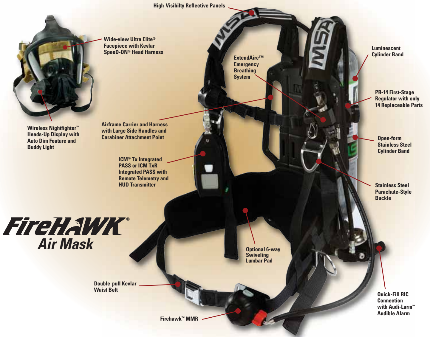
CBRN Compliant FireHawk ® Air Mask (NFPA 1981-2002 edition compliant, NIOSH 42 CFR Part 84 CBRN certified)
