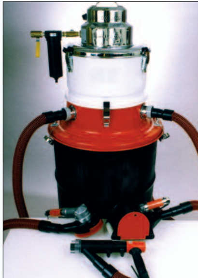
35/55 Gal. Dual Venturi 3 Port Vacuum 308.3350
