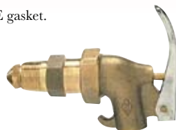
Part# 272037 - 1.40 lbs. Adjustable shank designed to easily adjust to proper drain position after installing in drum. Internal flame arrestor. FM APPROVED for use with oils (under 30 SAE) and non-corrosive flammables.
