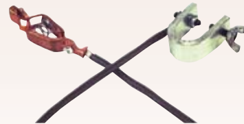
Part# 272032 - .64 lbs Deluxe Ground Wire: For connection between drum and true ground. Three-foot-long heavy duty insulated wire rope with "C" clamp on one end and alligator clip on the other.
