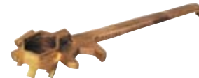
Part# 272086 (3 lbs.) Deluxe model. Built-in 1.25" wrench for tightening faucets into drums. Handles bung patterns 1, 2, 3, & 5.
