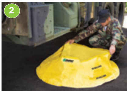
Step 2: Position Pool underneath spill source.
