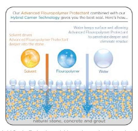
Innovative Hybrid Carrier Technology yields a unique solvent-based sealer that offers the highest level of protection and is V.O.C. compliant world-wide.
