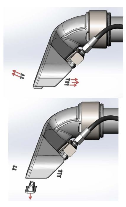
To replace the Glide, apply silicone sealant around the edge of the glide. Place the new Glide into the bottom of the wand head replace and hand tighten the five screws. If reattaching a glide that has already been used, lightly rotate the screws back and forth into the glide to find the original thread cut into the glide and hand tighten screws. Test the wand operation before returning to service.
