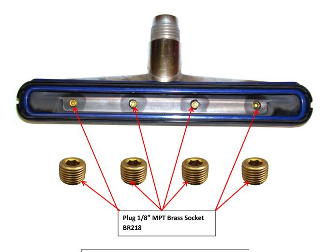
Use LOCTITE 545 THREAD SEALANT to seal the Brass Plugs screwing into the Cast Head
