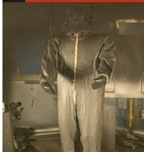
The Tychem® ThermoPro garment does not continue to burn after the flame exposure—maintaining a protective barrier to minimize burn injuries. (Image 3 seconds after flame source removed.)
