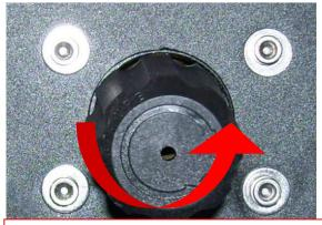
To decrease the solution pressure, turn the regulator/unloader knob counter-clockwise.
