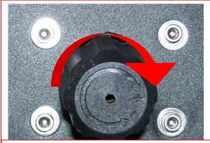
To increase the solution pressure, turn the regulator/unloader knob clockwise.
