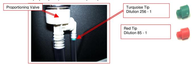
Metering Tip Kit (Hydro-Force Item# PDE001) contains 14 different colored metering tips, allowing dilution rates from 11:1 up to 427:1. Refer to the chart below to select the tip that meets the dilution rate for your chemical application.
