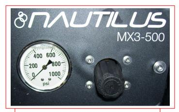
Pressure gauge & Regulator/Unloader
