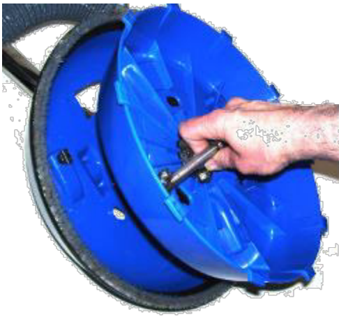
Retaining Nut Aligned for Inner Shell Removal
