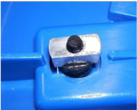
Retaining Nut Aligned for Inner Shell Removal
