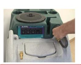
Place end of prime hose and use vacuum to prime the solution pump.
