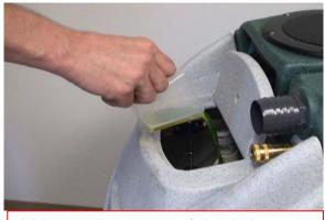
Add appropriate amount of chemical to water in solution tank
