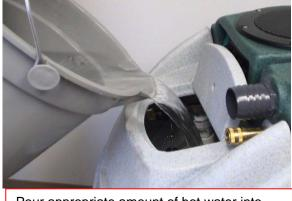
Pour appropriate amount of hot water into solution tank
