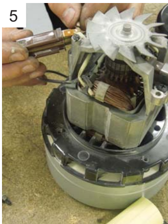
5 Remove brush from wire clip by sliding off groove. If brush is worn down to a length of 0.25" or less, replace brush.
