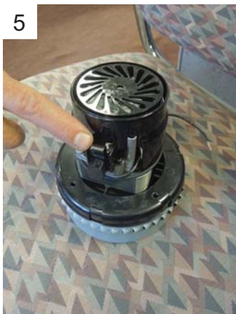
5 Remove the 2 metal motor-cap-retaining clips locating on each motor (for Amatec motors only)
