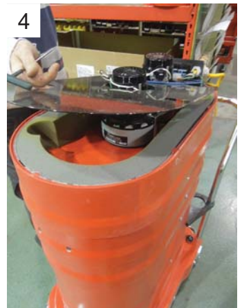
4 Lift motor shield up from deck to expose motors.
