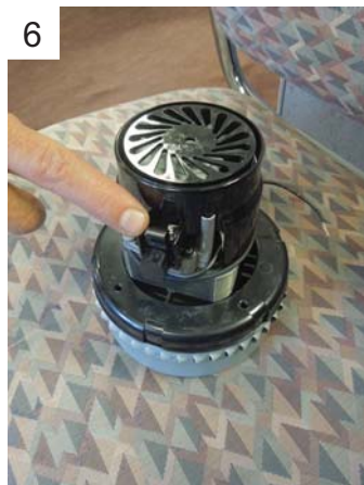
6 Remove the 2 metal motor-cap-retaining clips locating on each motor ( for Amatec motors only )
