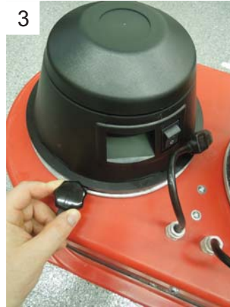
3 Loosen the motor retaining knobs enough to remove motor under negative pressure.
