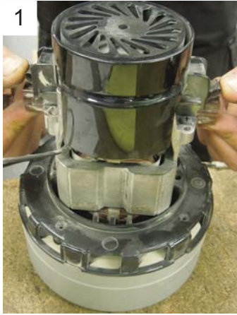
1 Remove motor fan cover by pressing down on clips located on each side.
