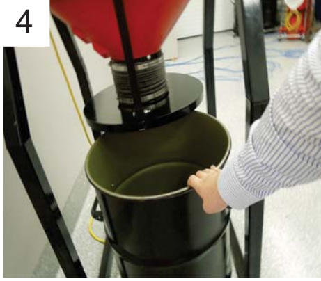
Once both pins and lid are locked in the up position, remove the drum by rolling the caddy unit from under the silo.
