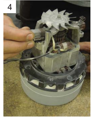
4 Pull brush out from wire clip.
