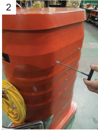
2 Disconnect hood from motor deck by removing 4 screws.
