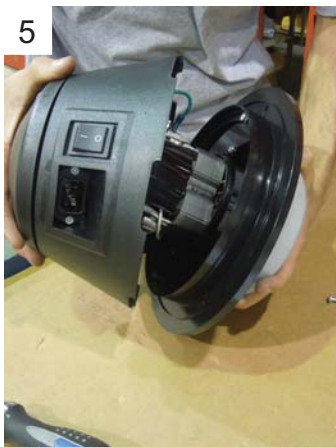
5 Remove the plastic motor cover to access the top of the motor.
