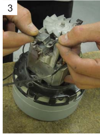
3 Repeat process for other side of brush.
