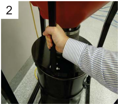
Once ball pin is released, pull up on the guide bar until it locks in the upward position, making sure the ball pin clicks into its designated hole.
