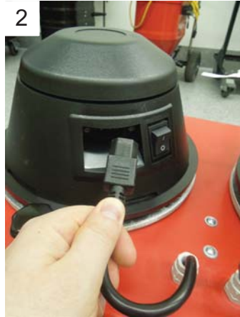
2 Disconnect motor terminal.
