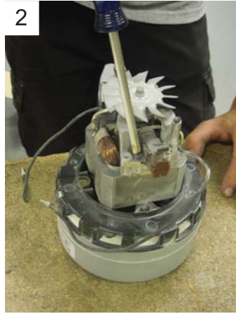
2 Remove both sets of screws located on one side of the brush.
