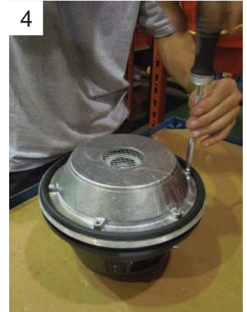
4 Remove the 6 screws attached to each motor assembly.
