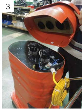
3 Remove silencer hood from motor deck.
